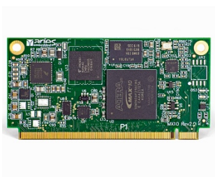
Image 2: For professional electronics designs in industrial applications, ARIES Embedded offers the MX10-SoM for Intel MAX®10-FPGAs.
