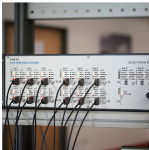
Image 2: The Automotive Ethernet Tester generates different traffic and speed grades and records them
