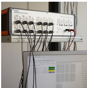
Image 1: The Automotive Ethernet Tester (AET) is a highly-automated test system for TC8 switching and AVB/TSN tests
