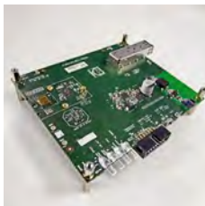
Image 2: Evaluation board included in the evaluation kit EVK9351AUT for 1000BASE-RHC automotive bridge
