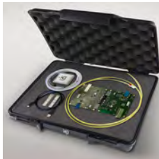
Image 1: Extensive evaluation kit EVK9351AUT from KDPOF eases project start for optical gigabit connectivity
