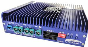
Image 1: Renesas implements KDPOF's 1000BASE-RHC optical physical layer in new vehicle computer VC4
